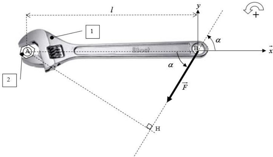
$$\{T_{main \rightarrow 1}\} = \left\{ \begin{array}{c} \overrightarrow{R_{main \rightarrow 1}} \\ \overrightarrow{M_{B,main \rightarrow 1}} \end{array} \right\}_B = \left\{ \begin{array}{c} \vec{F} \\ \vec{0} \end{array} \right\}_B$$
